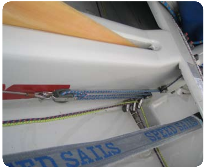
Standard modern arrangement using a combination of rope and wire
