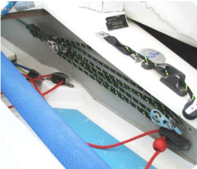
System retrofitted to series 2 Don Marine FRP boat.
